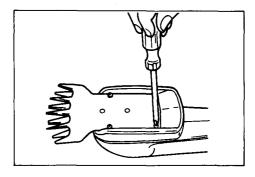
When installing the new blades, rotate the gear so that its ring is positioned in the blade guide hole. With the blades held in this position, replace the screws and tighten them securely.
